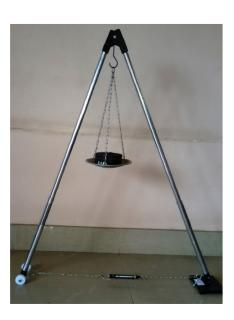
A metallic apparatus, about 1.2m in length whose one leg is fitted on an unmovable bracket and the other on rollers. Spring balances show tension on the rod and the compression on rafters. Apparatus is supplied complete with a dynamometer, chain and pan.
